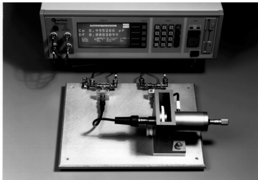
Figure1: QuadTech 7600 Precision LCR Meter connected to Dielectric Products LD-3 Cell
